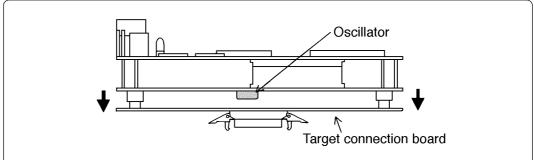
Apply an equal amount of force to the connectors on each end of the target connection board when pulling the board out. Note: Do not apply excessive force to the connectors. Excessive force can break the connectors.
